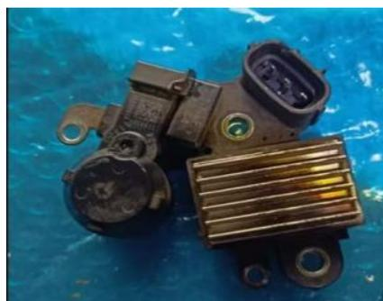
Gambar 2.8 Tampilan IC *Voltage regulator*
