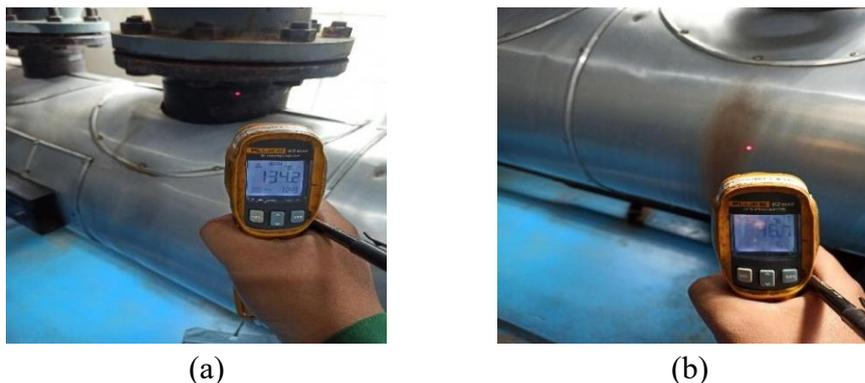
**Gambar 3.** Temperatur *in-situ* pipa *steam header*
